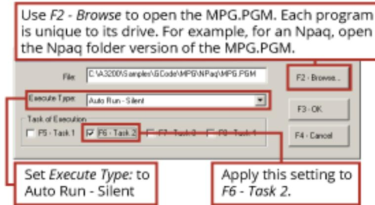
**Figure B-31: Configure Program Automation (MPG.Pgm)**
