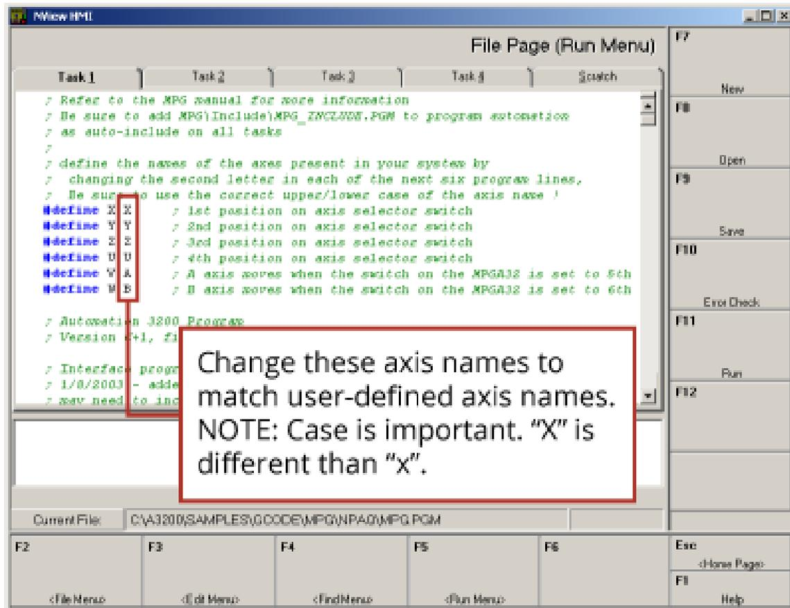
**Figure B-23: Assigning Axis Names**
