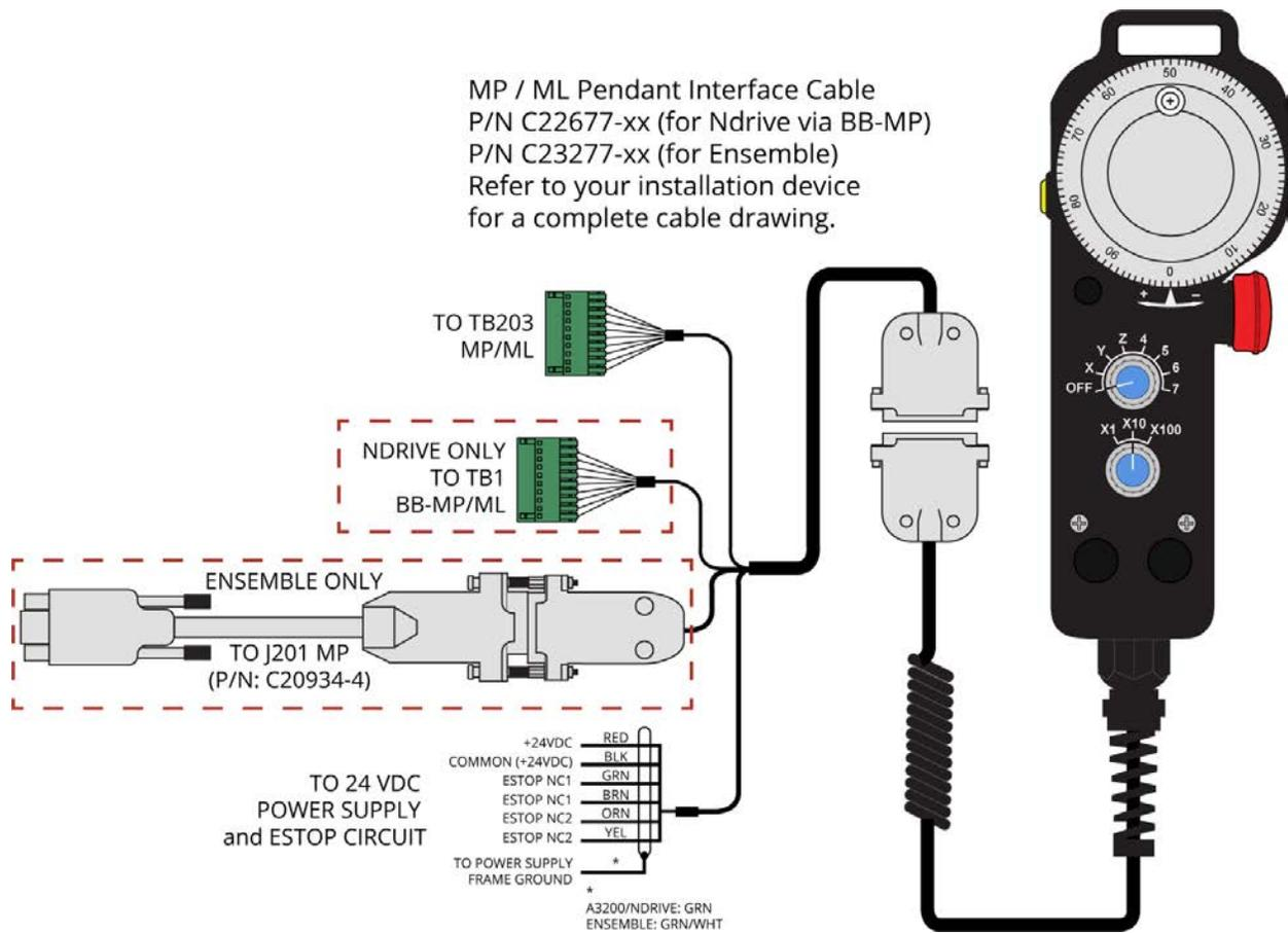
Figure B-3: MPG to MP/ML Cable Drawing
