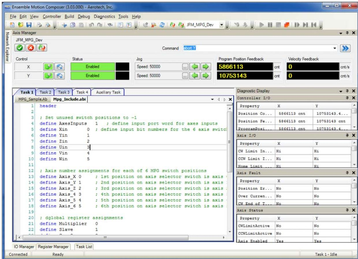
**Figure B-39: Assigning Axis Names**
