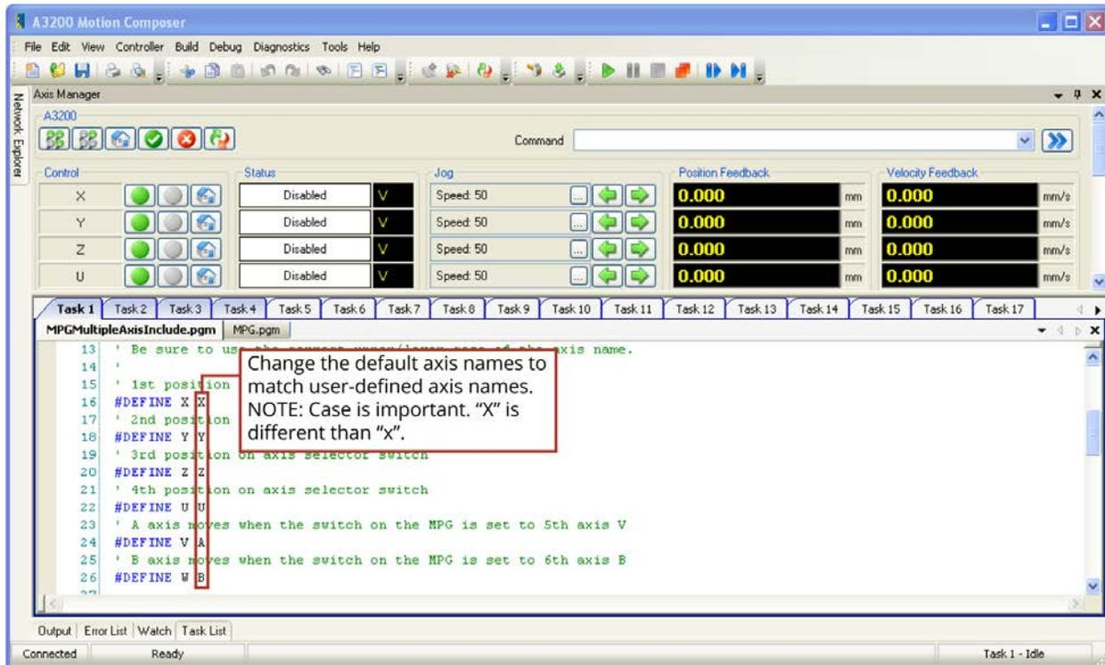
**Figure B-11: Assigning Axis Names**
