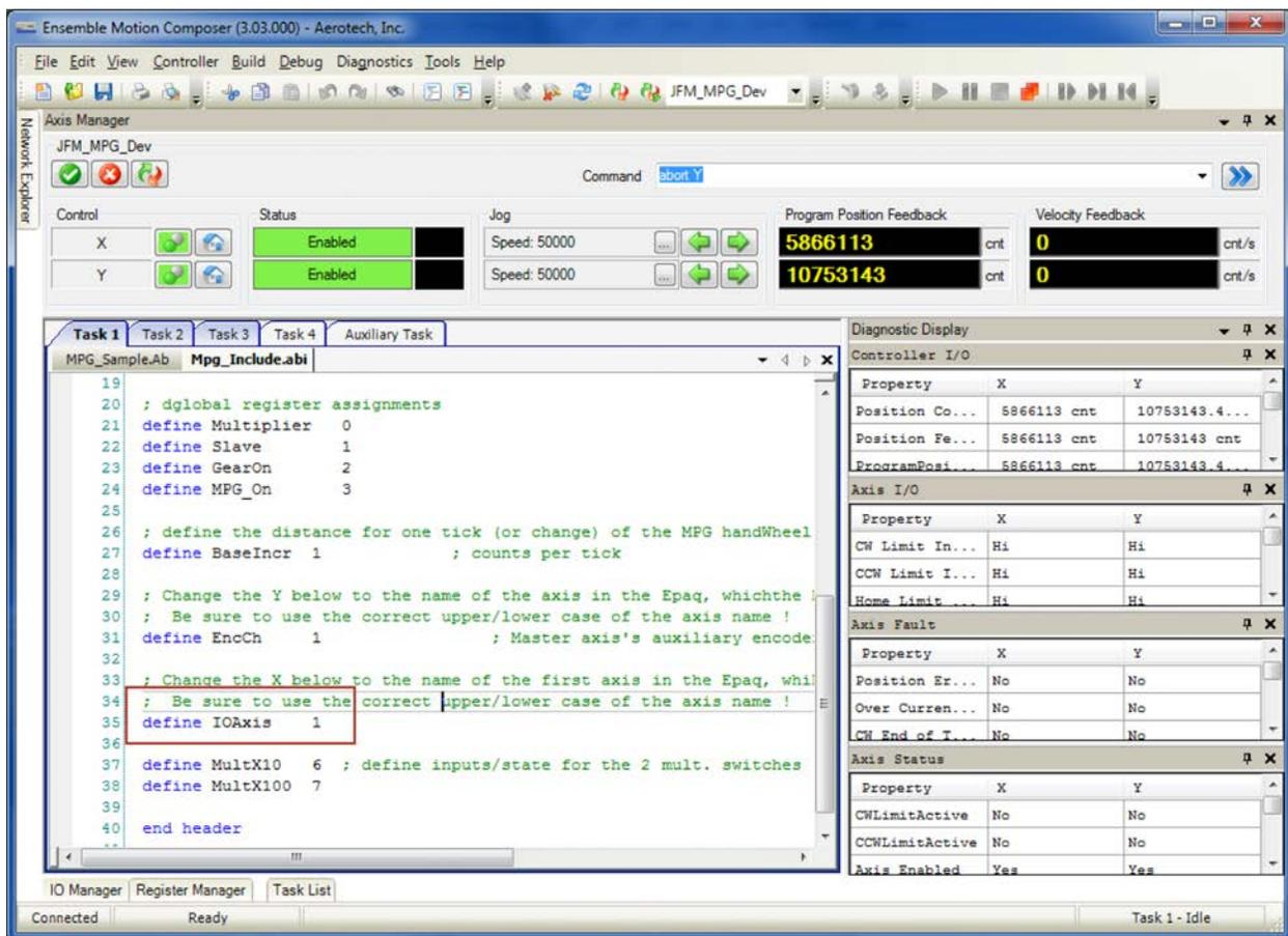
**Figure B-42: Defining the MPG I/O Connection**
