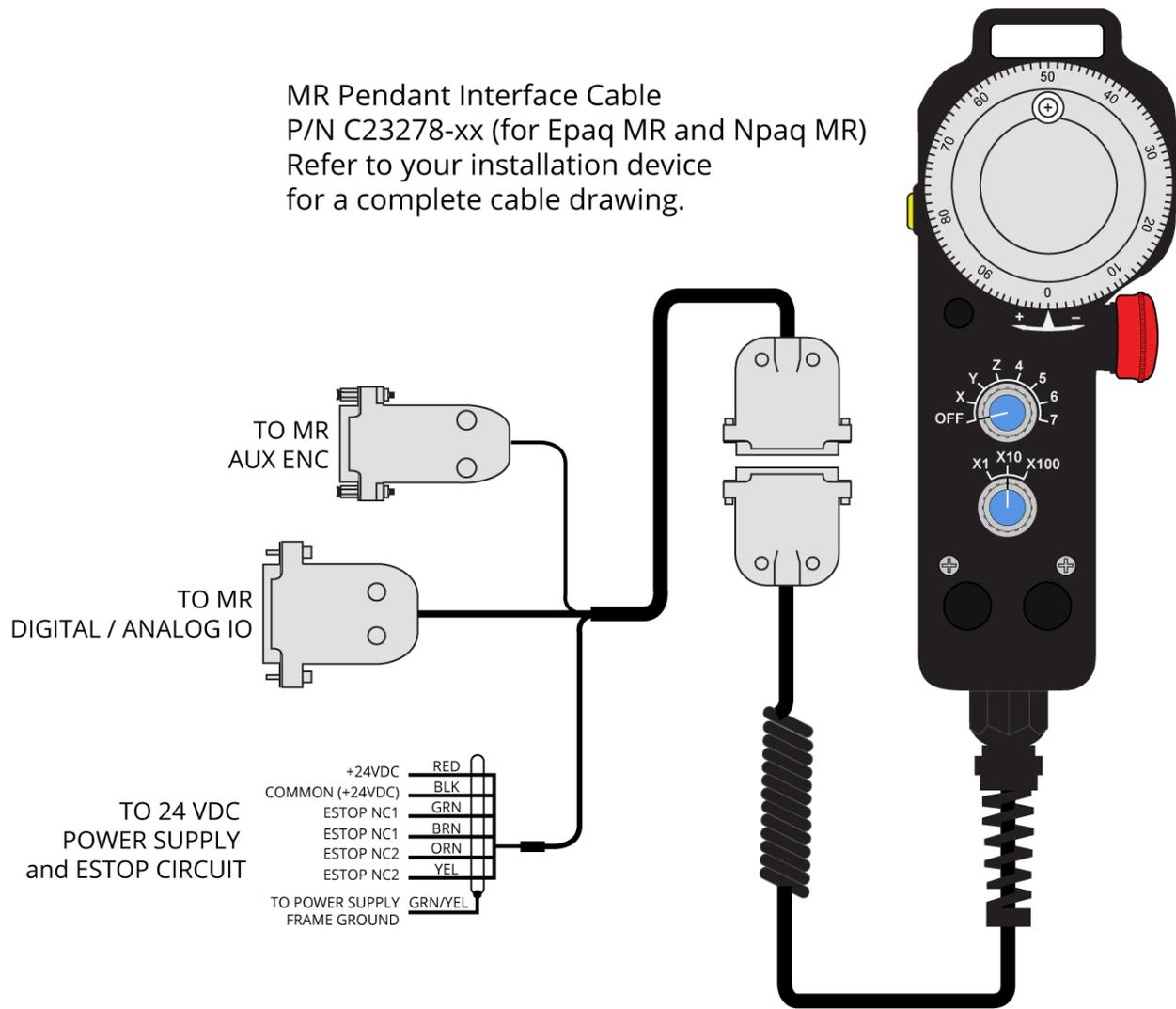
Figure B-7: MPG to Epaq MR/Npaq MR Cable Drawing
