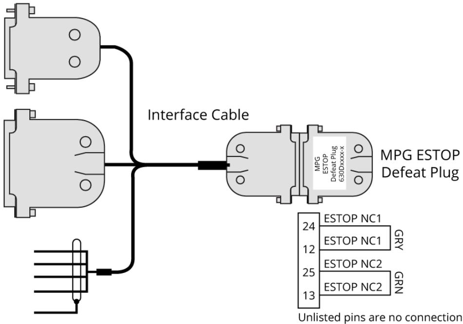
**Figure 2-3: Bypass Plug**
