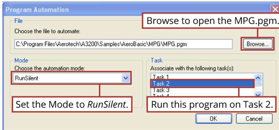
**Figure B-18: Configure Program Automation (MPG.Pgm)**
