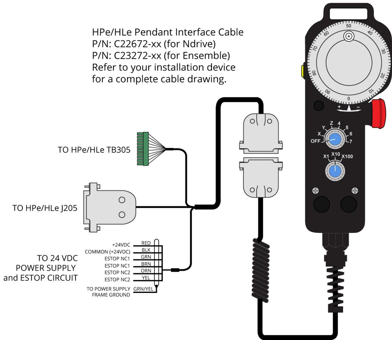
**Figure B-1: MPG to HPe/HLe Cable Drawing**
