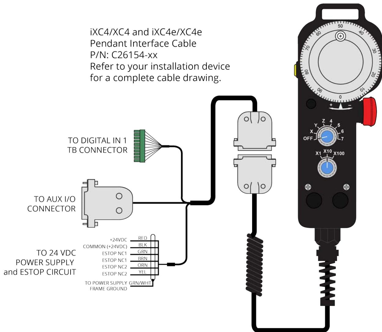
**Figure 2-4: MPG to XC4/XC4e Cable Drawing**
