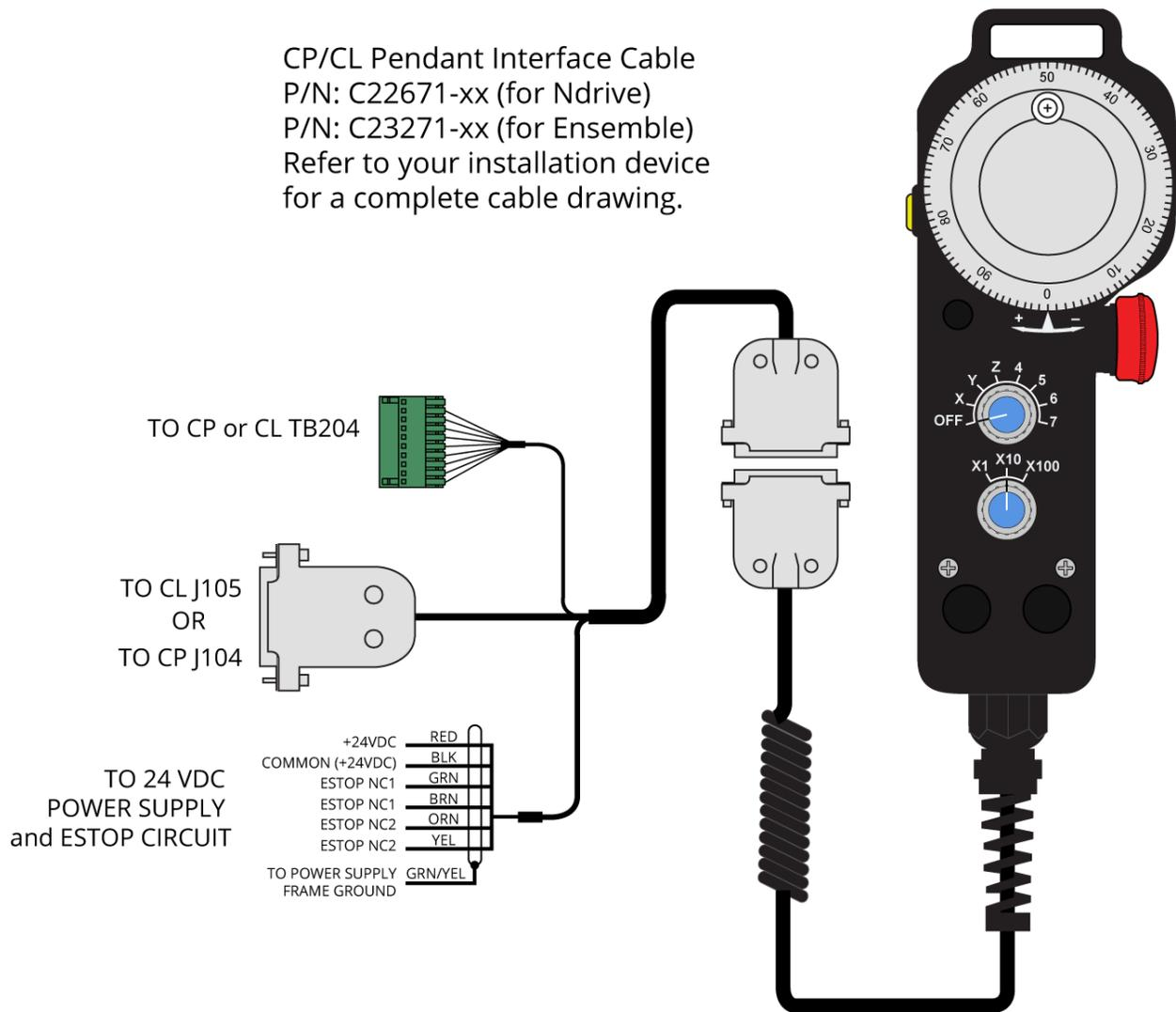
Figure B-2: MPG to CP/CL Cable Drawing
