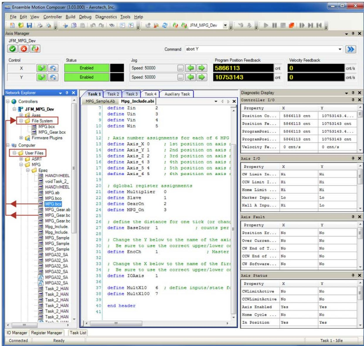
**Figure B-44: Copying Files to the Controller**
