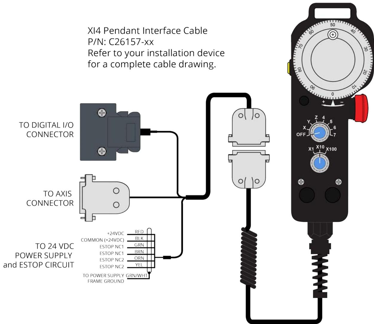
Figure 2-6: MPG to XI4 Cable Drawing
