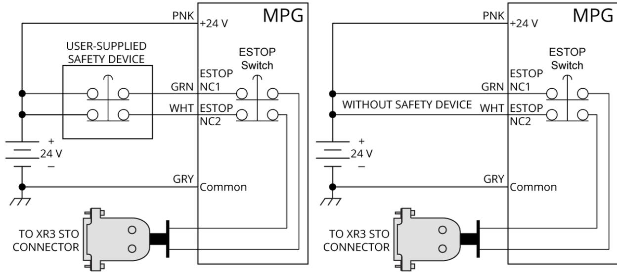
**Figure 2-9: Automation1 XR3 Safety Device Connection Detail**
