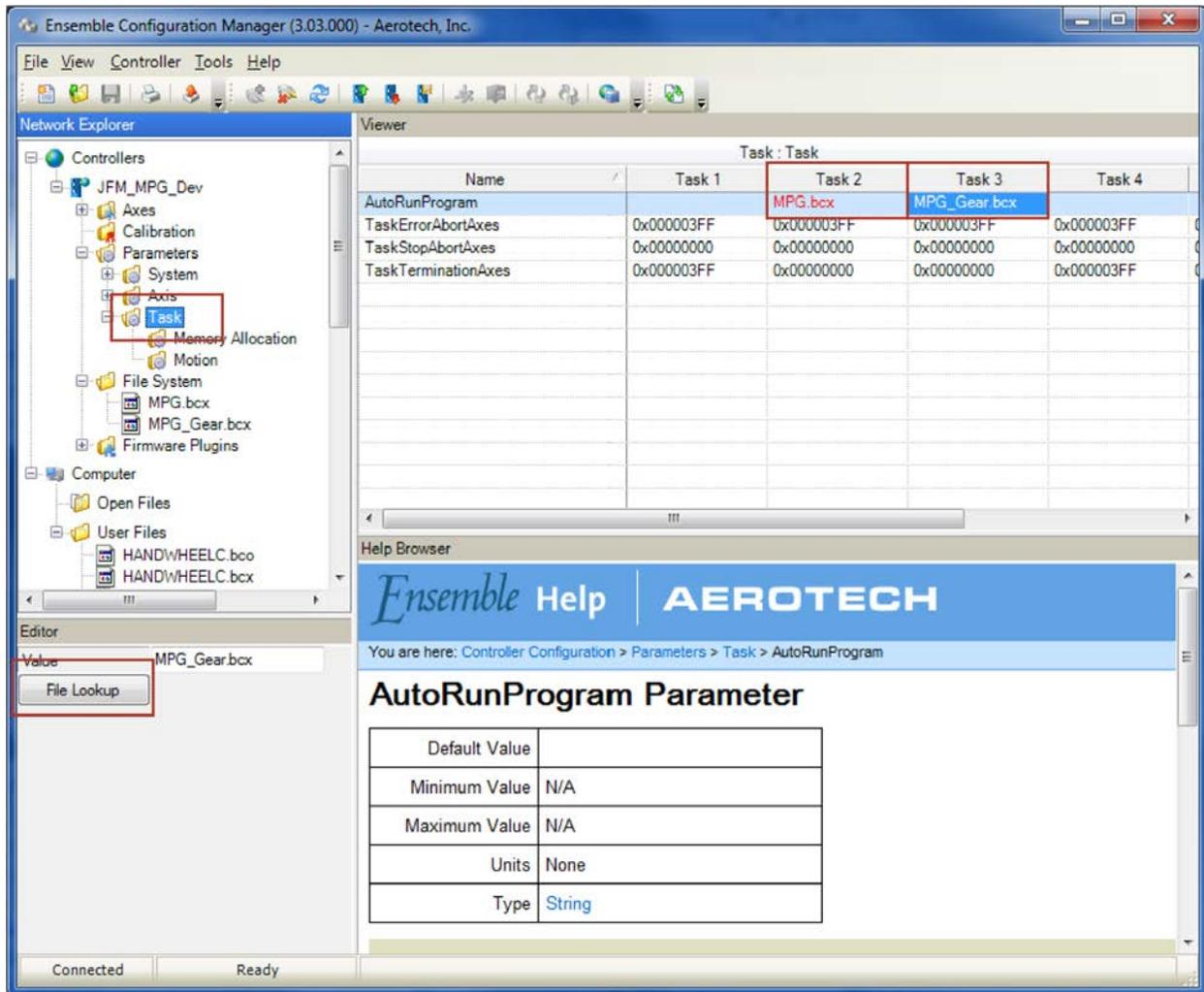
**Figure B-46: Select the Auto-Run Task parameters**
