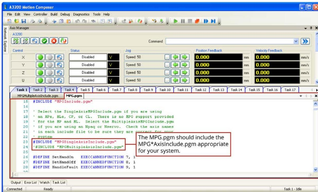
Figure B-10: Set the Correct Include File
