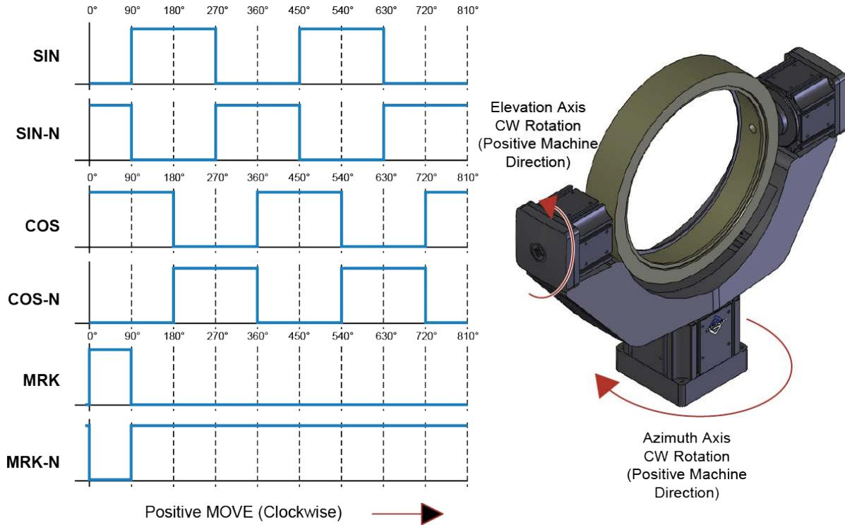
**Figure 3-5: Encoder Phasing Reference Diagram (Analog/Sine Wave)**
