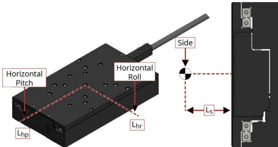
**Figure 2-5: Cantilevered Load Capabilities**
