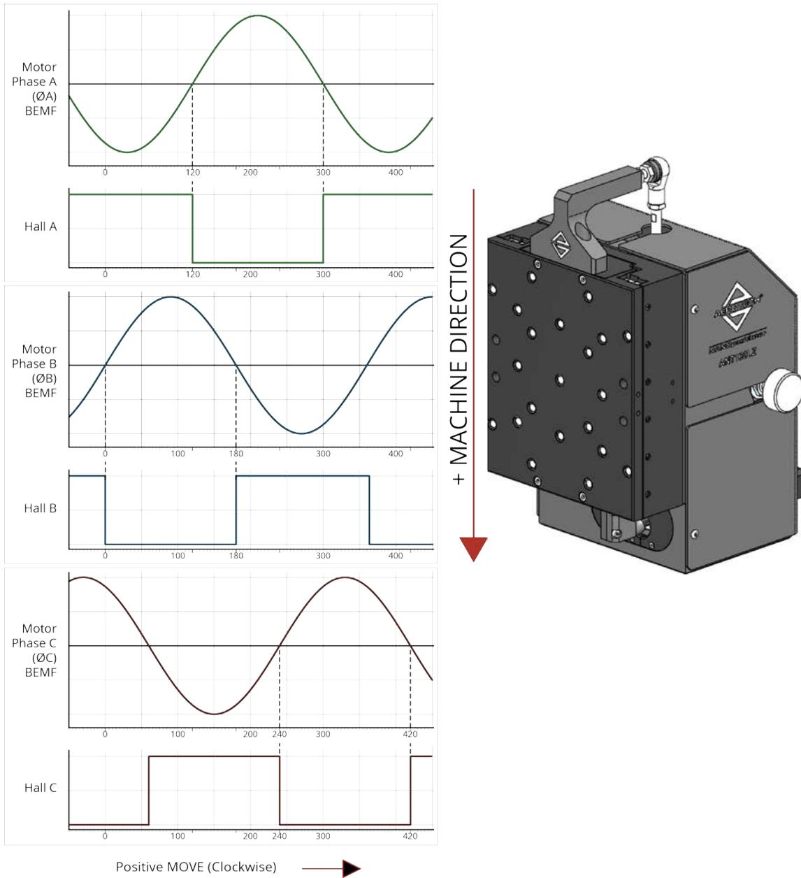
**Figure 3-5: Encoder Phasing Reference Diagram (Standard/Square Wave)**
