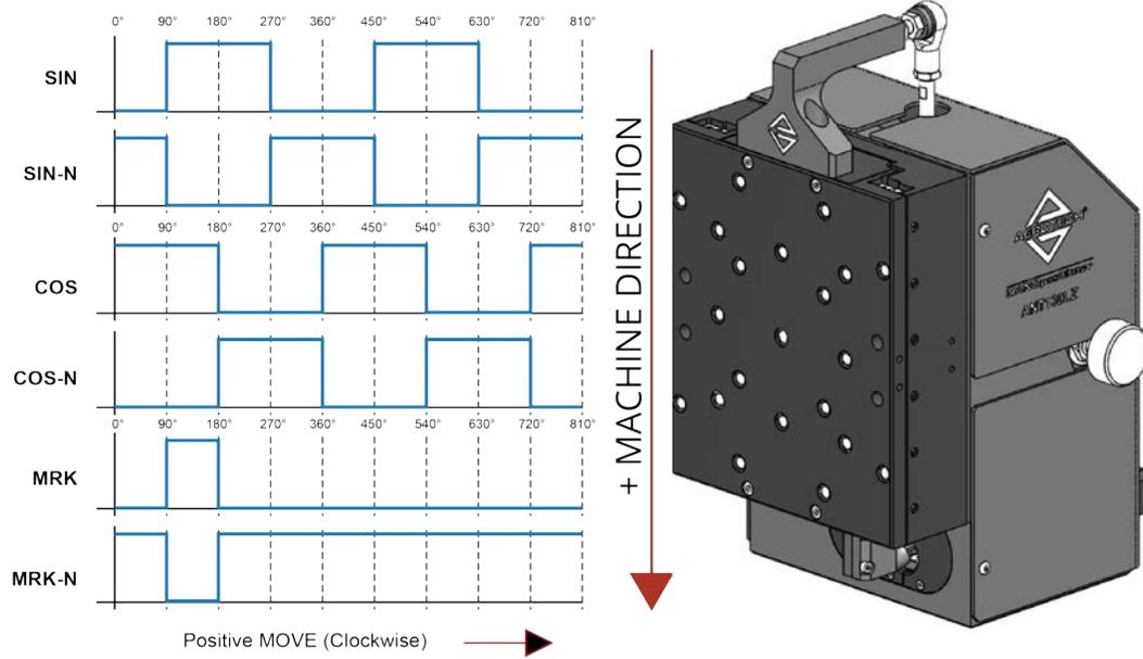
**Figure 3-6: Digital Encoder Phasing Reference Diagram (Sine Wave)**
