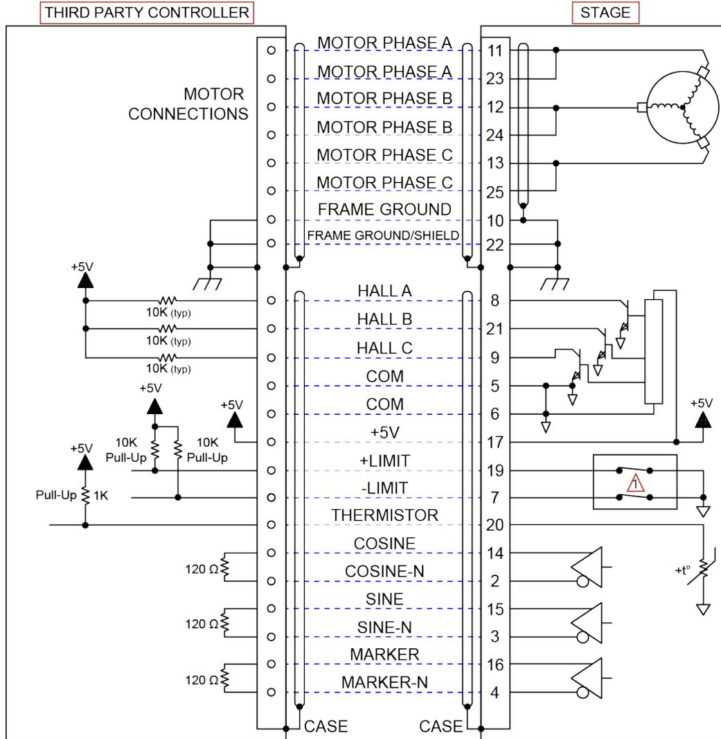
Figure 3-2: ANT130LZ Motor and Feedback Wiring [-CN2 Option]
