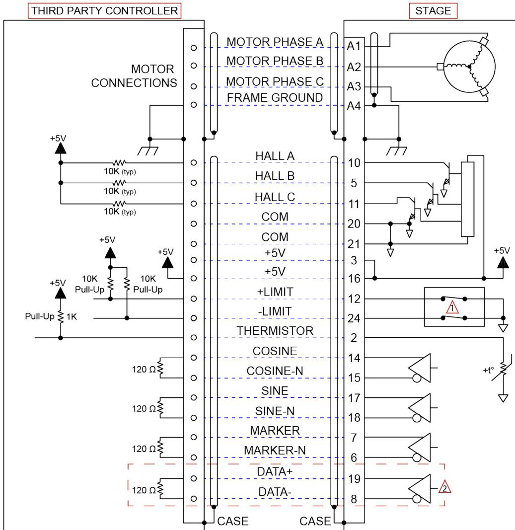
△ Over-travel limit switches are normally-closed. △ -E3 encoder option only
