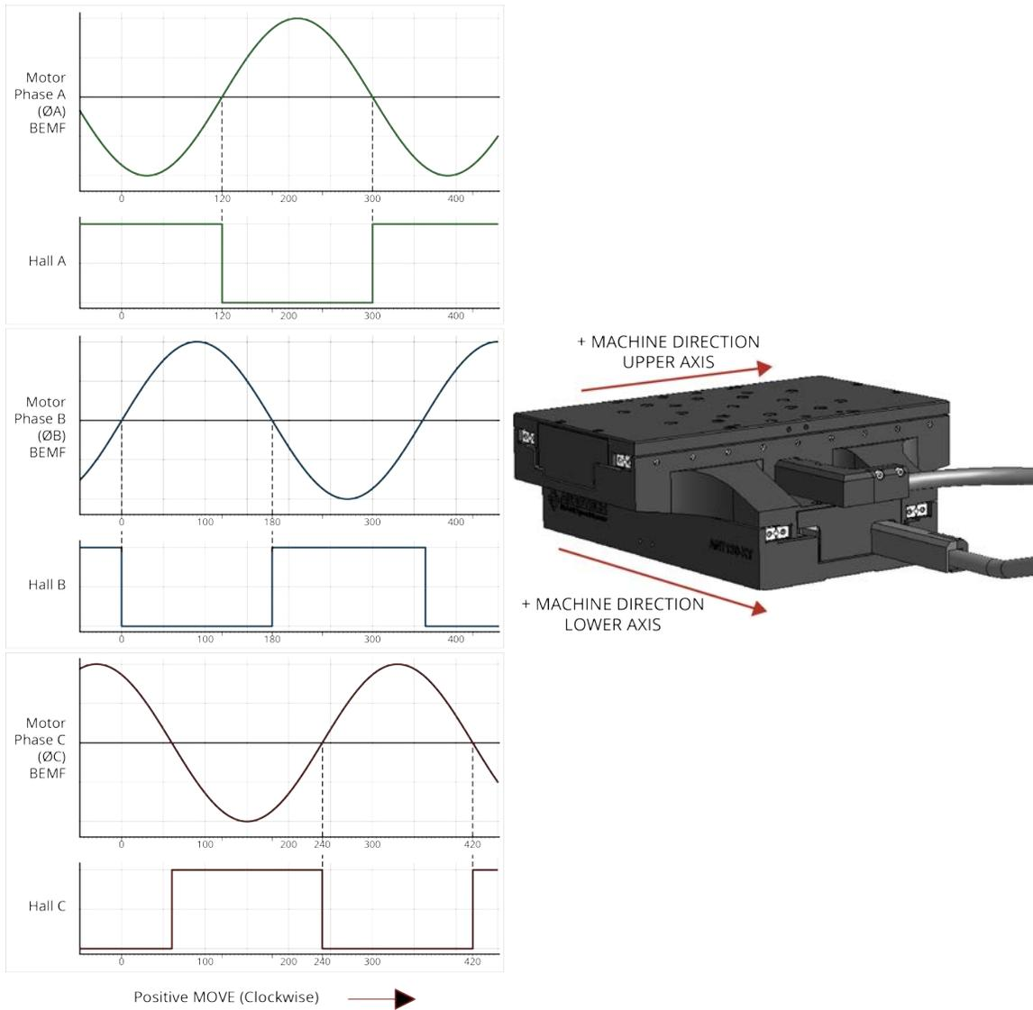
**Figure 3-5: Encoder Phasing Reference Diagram (Standard/Square Wave)**
