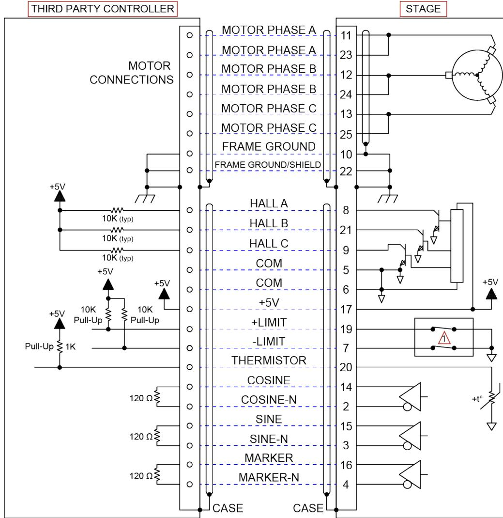
Figure 3-2: ANT130XY Motor and Feedback Wiring [-CN2 Option]
