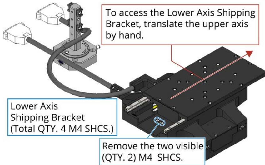
**Figure 6: Shipping Bracket Removal Procedure (Step 3)**
