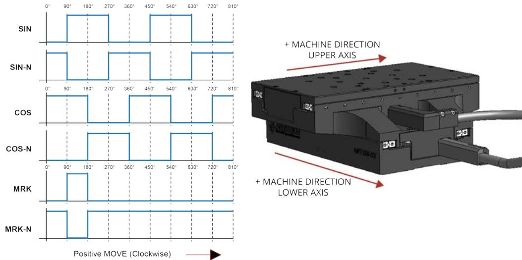
**Figure 3-6: Digital Encoder Phasing Reference Diagram (Sine Wave)**
