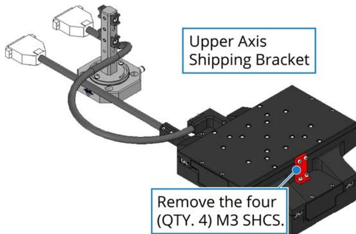
**Figure 5: Shipping Bracket Removal Procedure (Step 2)**
