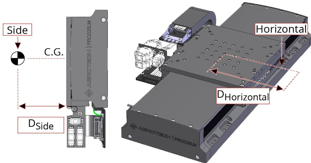
**Figure 2-4: Cantilevered Load Capability**
