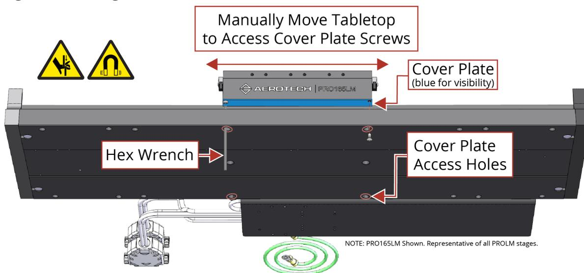
**Figure 4-8: Manual Feed Method**
