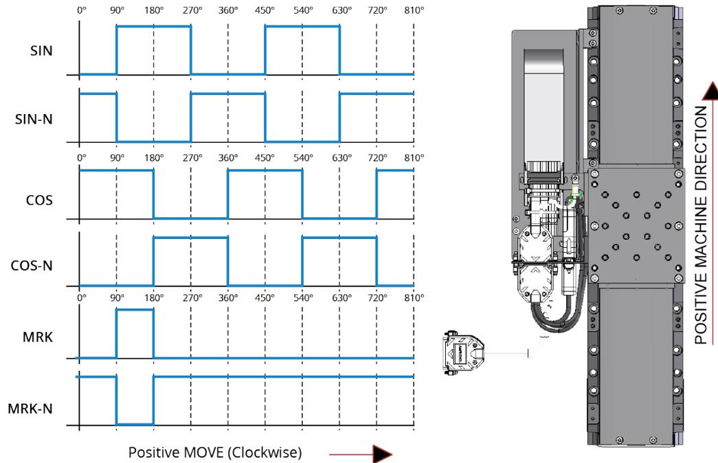
**Figure 3-7: Digital Encoder Phasing Reference Diagram (Sine Wave)**
