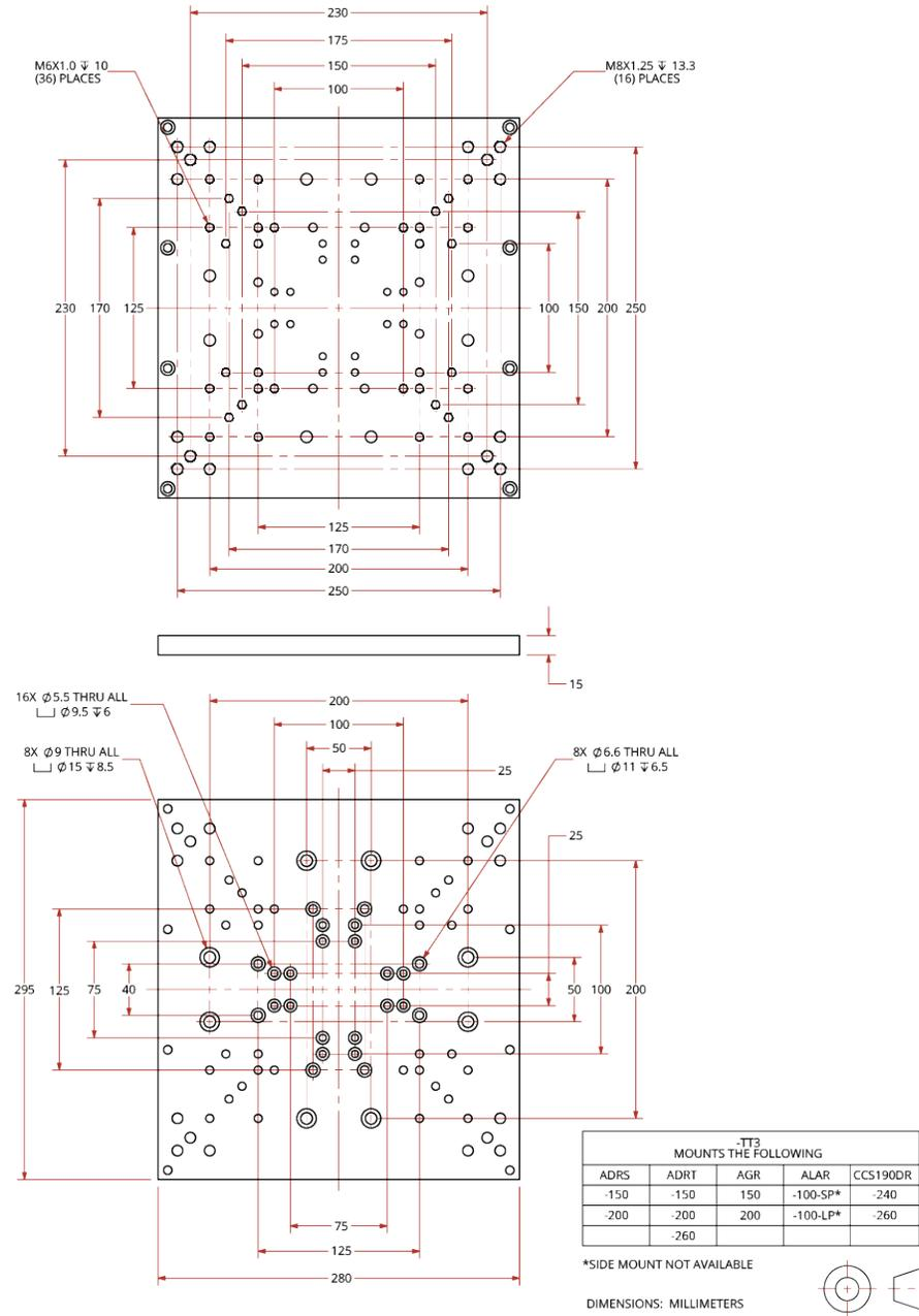
Figure 2-5: Z-Axis Bracket Dimensions
