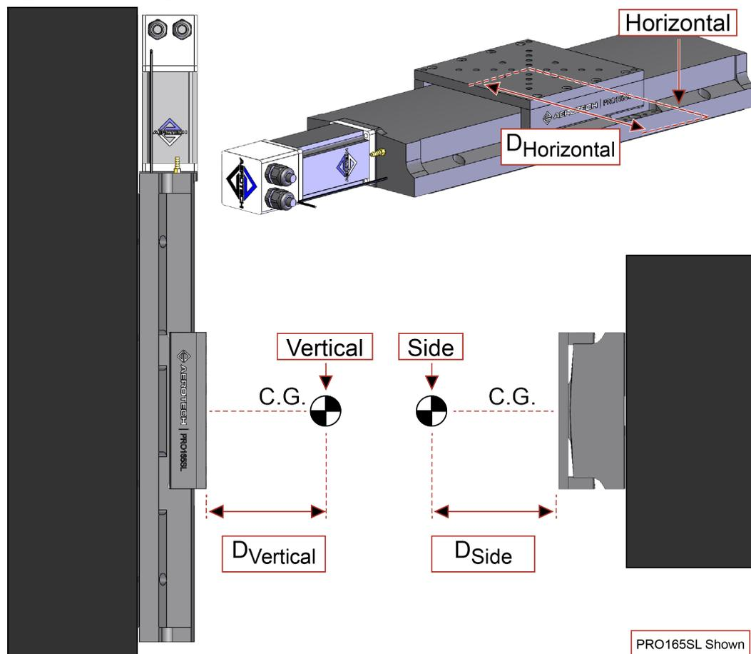
**Figure 2-7: Cantilevered Load Capability**
