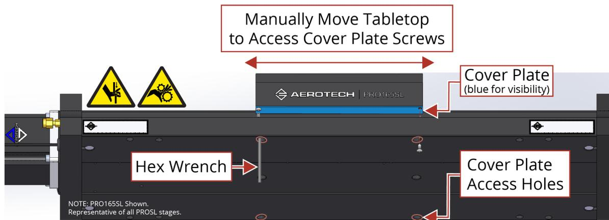
**Figure 4-12: Manual Feed Method**
