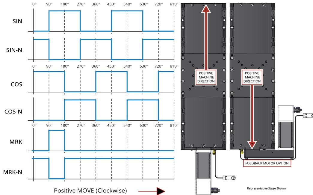
**Figure 3-6: Digital Encoder Phasing Reference Diagram (Sine Wave)**
