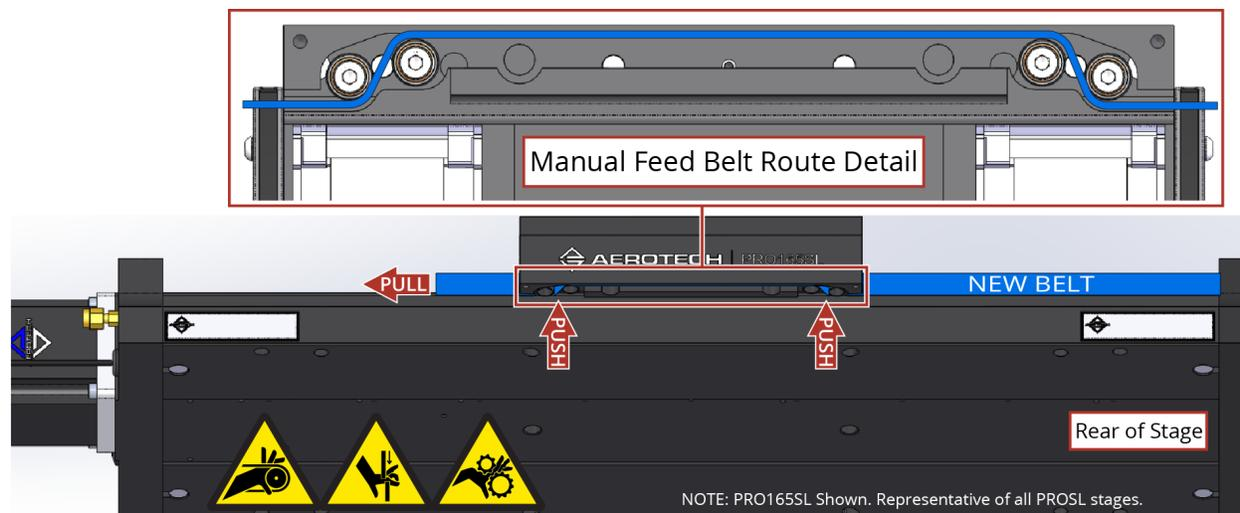
6. Manually pull the new belt back and forth through the table. Confirm that the side seal belt feeds through smoothly without friction or snagging. If there appears to be damages preventing successful installation, contact Aerotech Global Technical Support .
