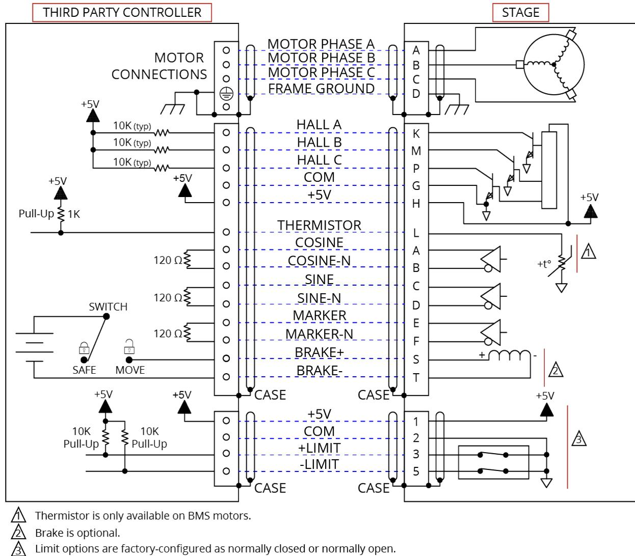
Figure 3-2: Brushless Motor and Feedback Wiring [-SLE Option]
