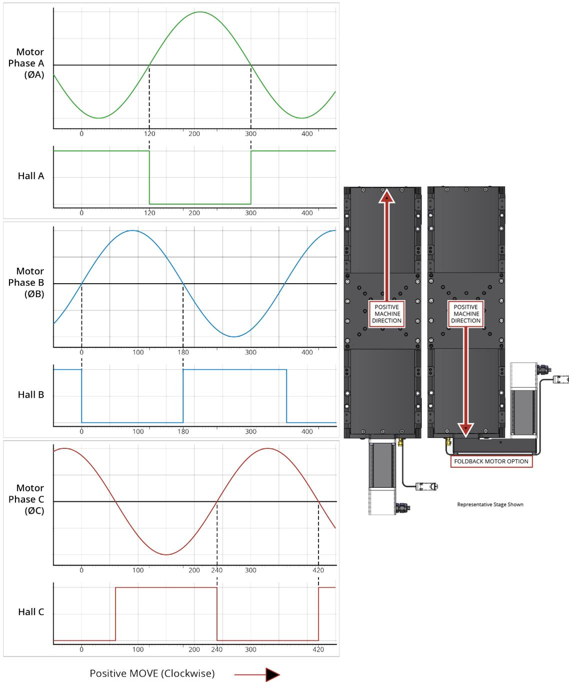
**Figure 3-5: Encoder Phasing Reference Diagram (Standard/Square Wave)**
