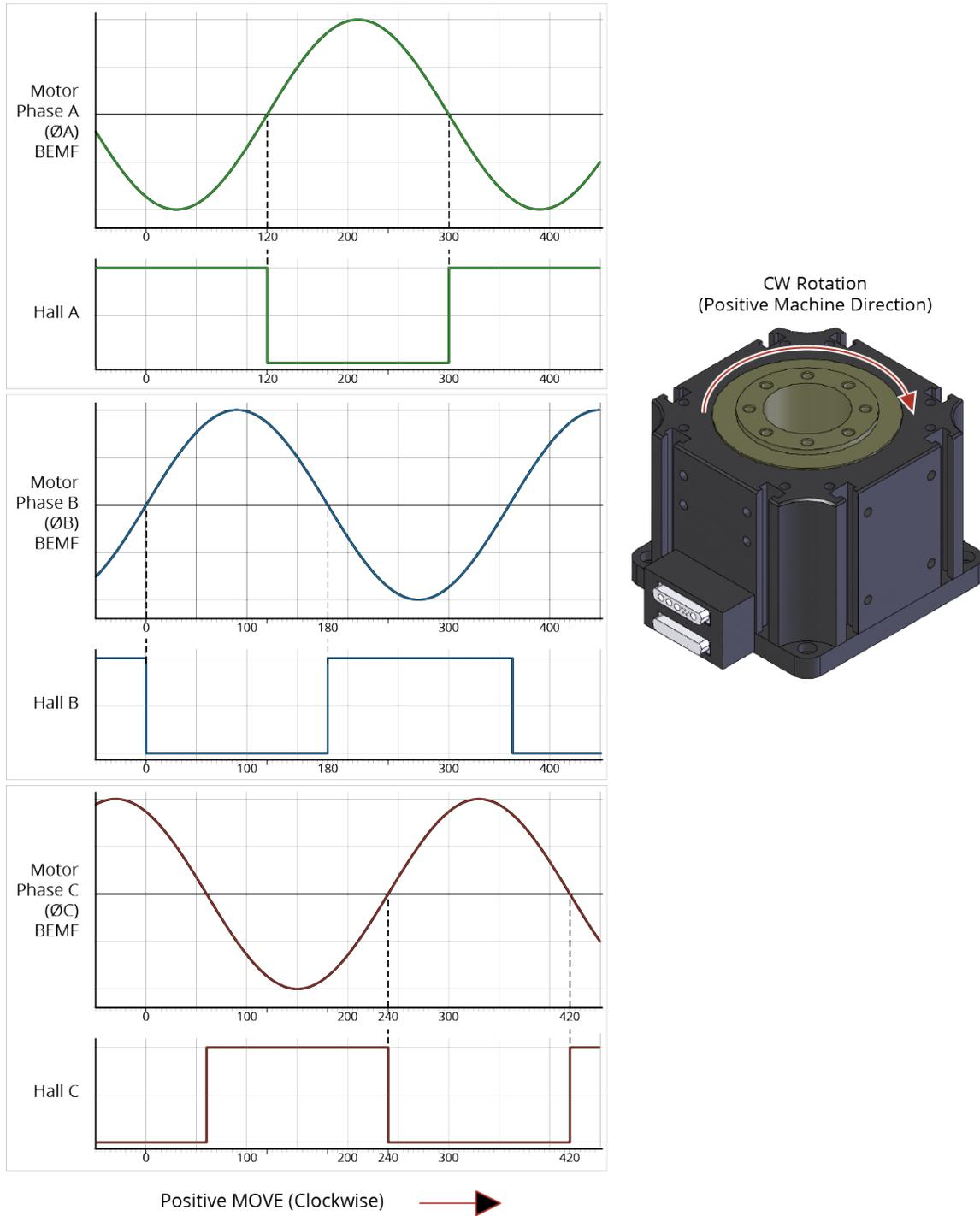
**Figure 3-4: Encoder Phasing Reference Diagram (Standard/Square Wave)**
